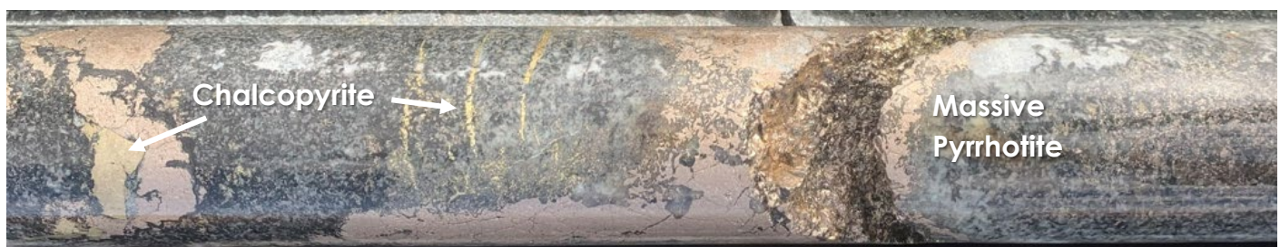
Figure 15. Massive sulphides in TMDD0001, chalcopyrite, pyrrhotite and pyrite observed, 841m depth.
