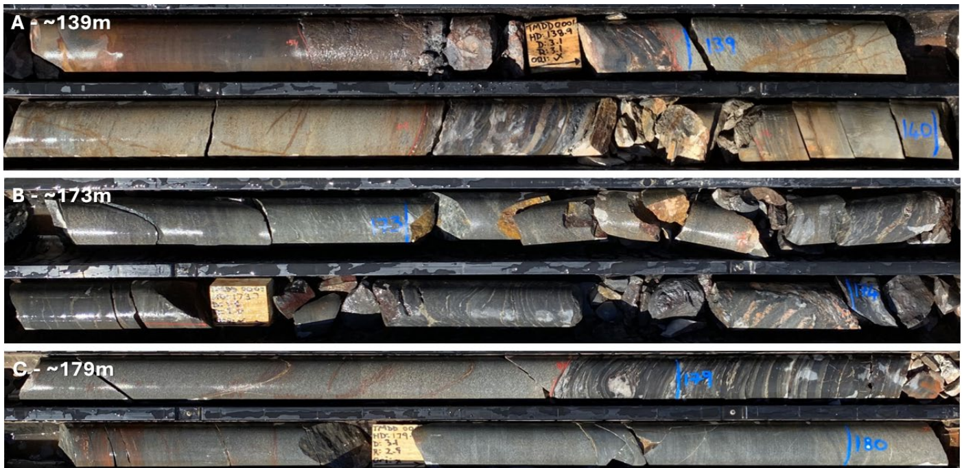
Figure 12. Diamond core photographs of the iron-rich sediments of the Dead Bullock Formation (DBF). A) At approximately 139m, folded iron-rich sediments of the DBF. B) Folded siltstone and shale units of the DBF at ~173m, with multiple folding and shearing events overprinted, with k-feldspar alteration. C) Sediments of the DBF, with increased pyrite and quartz veining. Refer ASX releases 1 December 2022 and 25 October 2022.
