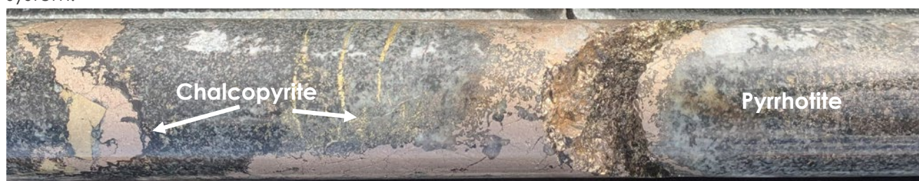
Figure 17. Massive sulphides in TMDD0001, chalcopyrite, pyrrhotite and pyrite observed, 841m depth 7,13 .
