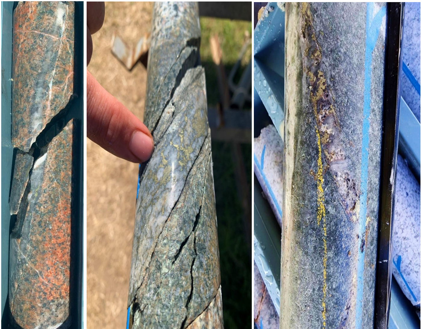
Figure 8. Left to Right. MRDD001, 227.3m strong potassic alteration of granodiorite with sulphide bearing quartz-vein (0.6m @ 10ppb Au, 0.5g/t Ag & 857ppm Cu). MRDD002, 136.15m quartz-sulphide vein within shear of strong sericite alteration of granodiorite (0.5m @ 9.35g/t Au, 21.1g/t Ag & 0.7% Cu). MRDD003, 34.9m strong silica and sericite alteration in granodiorite, quartz veins with visible chalcopyrite (0.6m @ 0.3g/t Au, 37g/t Ag & 1.6% Cu). (Refer ASX Announcement 21 October 2024)
