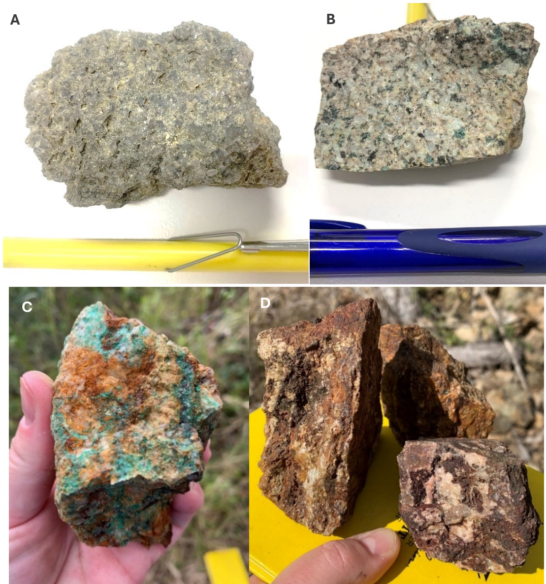
Figure 3. Host Rocks found at the Kaa Prospect. A) Strongly magnetic mica-rich breccia rock found at top of the Kaa prospect, representing the top of a breccia pipe. B) Wonbah Granodiorite. C) Sample MRRK071, 3.49g/t Au, 2.8% Cu & 195g/t Ag. D) Sample MRRK072, 6.06g/t Au, 585g/t Ag, 1.5% Cu, and 3.58% Sb (Refer -ASX Announcement 9 July 2024).
