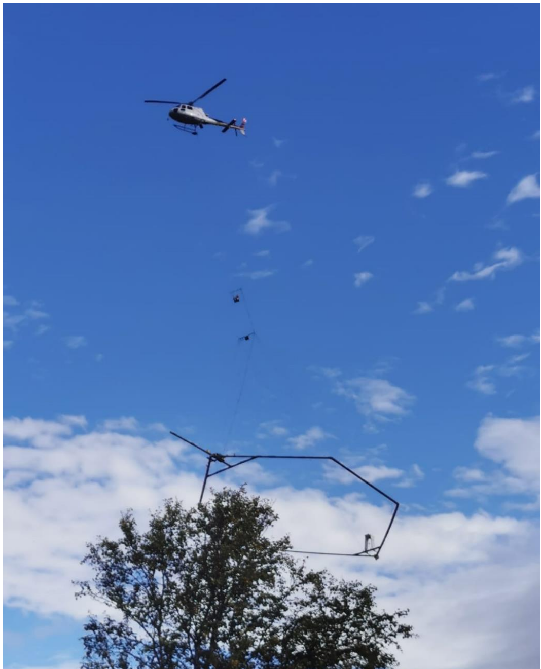
Figure 1: SkyTEM Airborne Geophysical Survey over Vangrøfta Copoer Project
