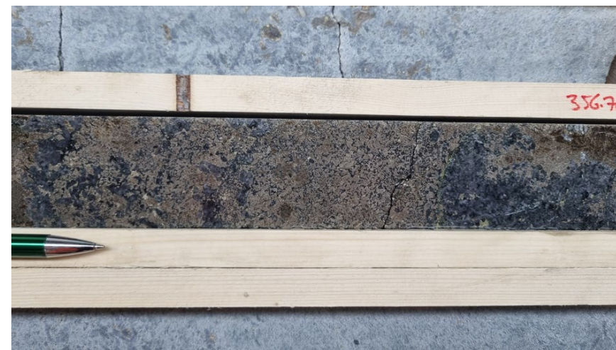
Plate 4: Massive pyrrhotite-pentlandite-chalcopyrite hosted by medium grained pyroxenite from a 0.54 m sample that returned 3.7% Ni, 0.20% Cu, 0.15% Co from 361.0 m, KUSK0015 (RTX drilling).
