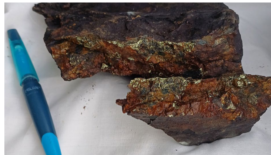
Plate 2: Chalcopyrite-quartz vein hosted in paragneiss. 4.4% Cu, 0.01% Ni, 1.8 g/t Au, 0.50 g/t Pd, 0.06 g/t Pt. Viridnechokka area, sample 14508.
