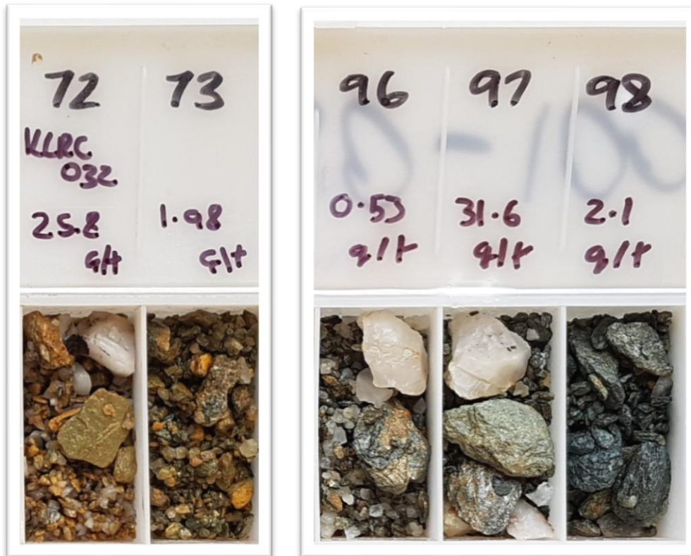
Figure 5: (Left) Partially weathered talcose/chloritic ultramafic schists with quartz veining and minor sulphides in RC chips from hole KLRC032 (2m @ 13.88 g/t Au from 71m). (Right) fresh talcose/chloritic ultramafic schists with quartz veining and sulphide (3m @ 11.39 g/t Au from 95)
