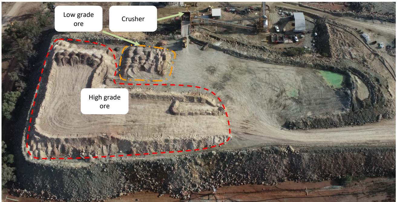
Figure 4: Stockpiled oxide ore on the ROM pad.
