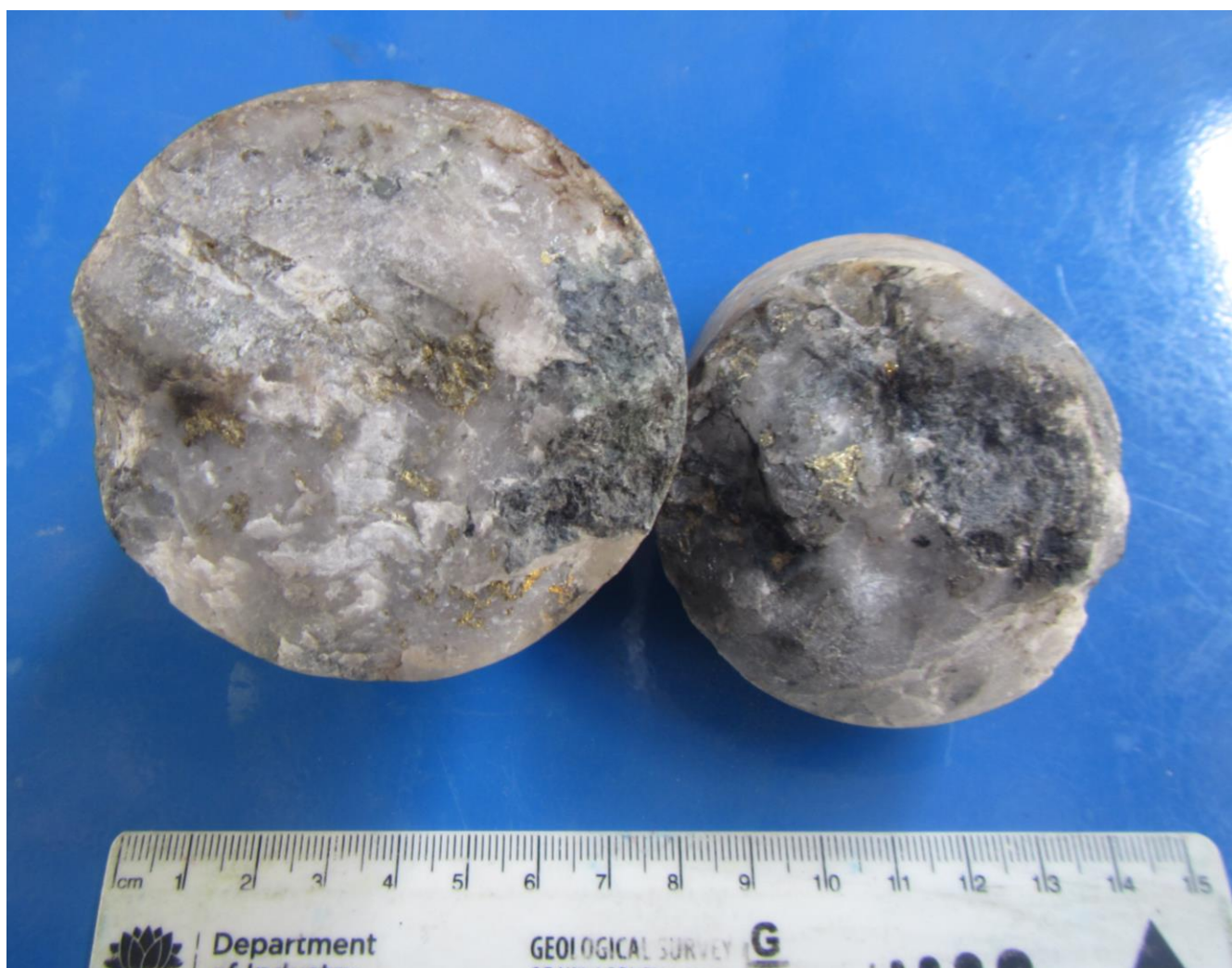
Figure 1 - Core from 114.5 m depth featuring chalcopyrite and chlorite in quartz veining
