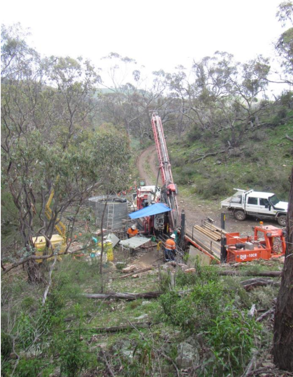
Figure 2: Diamond Drilling at Dead Horse Reef, QRD005
