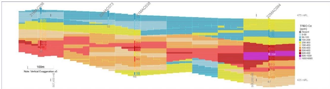
Figure 3 Section 7171519N showing Block Model grade distribution
