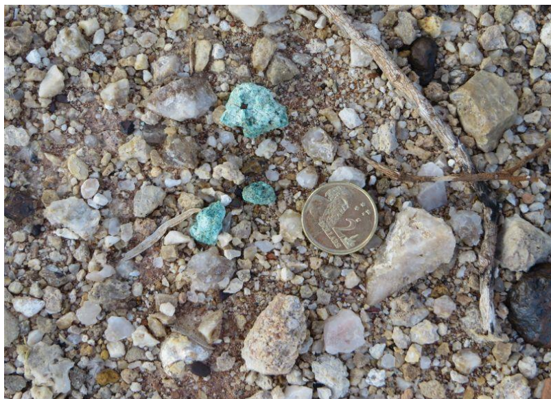
Figure 6: Malachite mineralisation in silicified dolomite drill cuttings – Cork Tree Prospect
