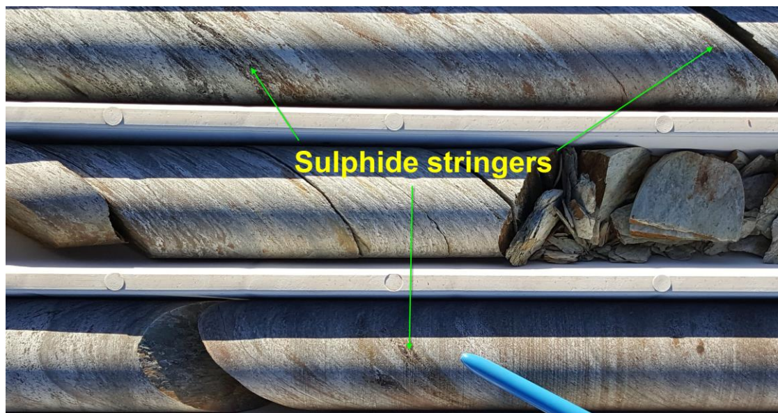
Figure 5: Existing diamond drill core with uncut disseminated (stringer?) base metal mineralisation from the Conquistador Prospect
