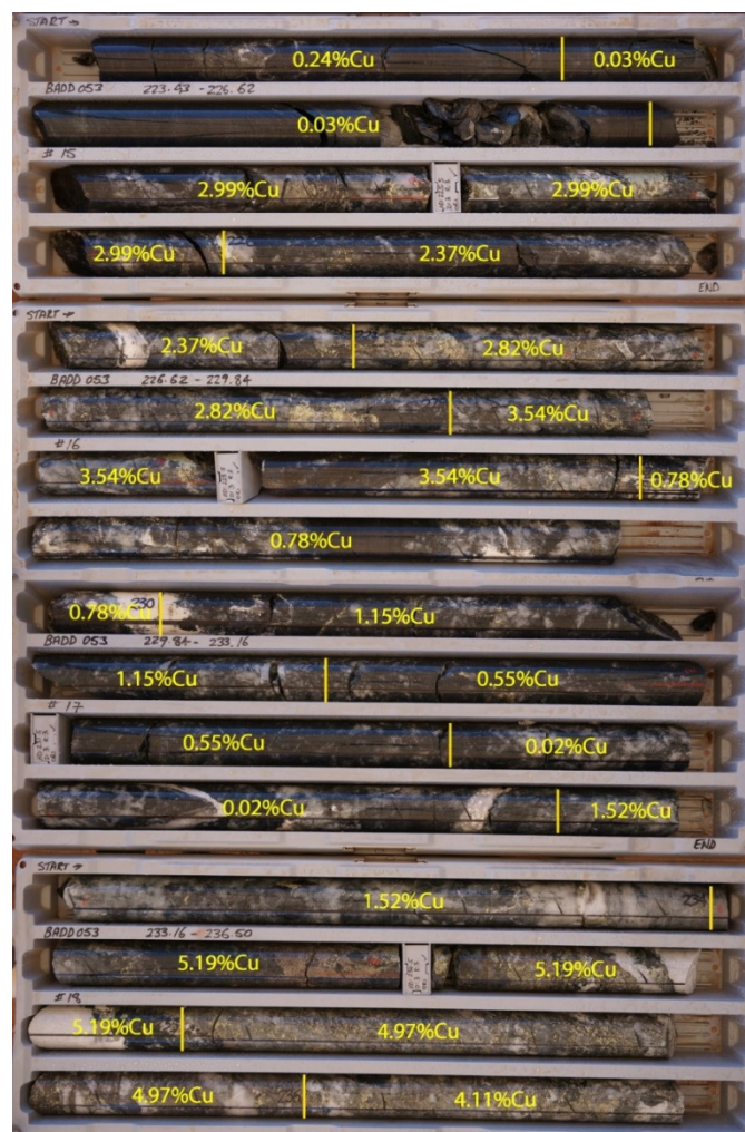
Figure 5 – High grade copper (coarse grained chalcopyrite) mineralisation in BADD053. Mineralisation associated with sheared quartz – carbonate veining and biotite schist in the Hangingwall Lode position is illustrated. Chalcopyrite mineralisation development from 225 to 257.5 metres downhole. True width is approximately 85% of downhole width.
