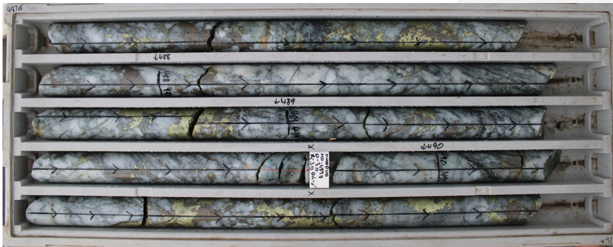
Figure 5. Chalcus Lodge in MHDD110 487m-491m showing strong chalcopyrite (yellow) and pyrrhotite (brown) mineralisation.
