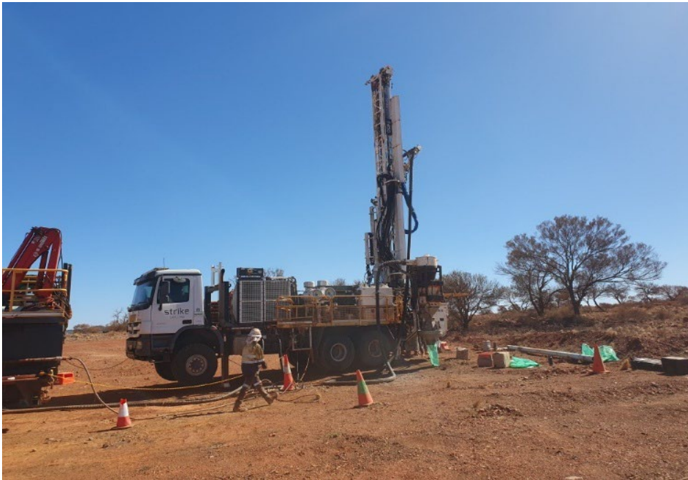
Photo 1: RC Drilling rig on site at Red Dog, Laverton Gold Project
