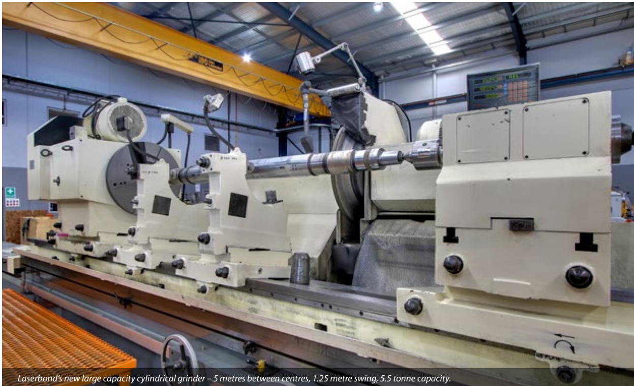
Laserbond's new large capacity cylindrical grinder – 5 metres between centres, 1.25 metre swing, 5.5 tonne capacity.
