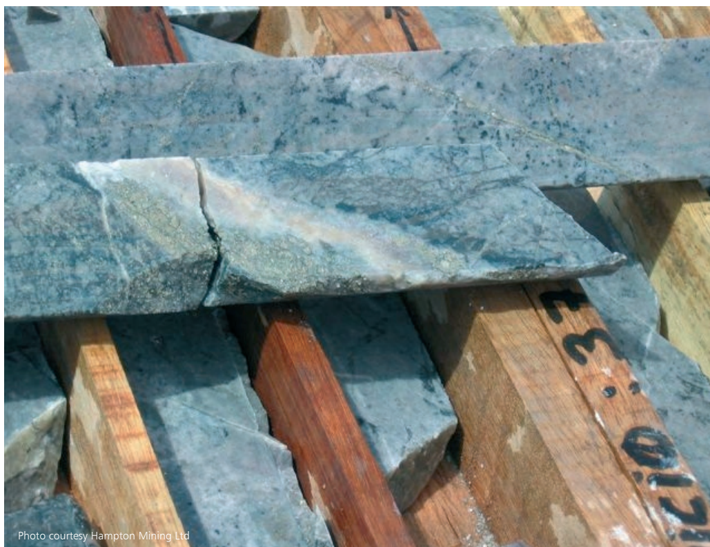
Los Calatos diamond drill core showing typical porphyry style alteration and sulphide mineralisation
