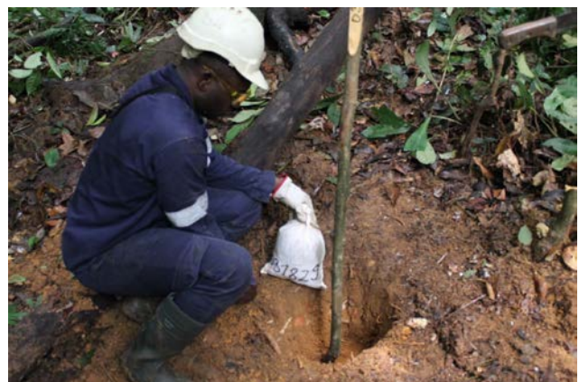
Photos 1 & 2: Stream Sediment and Soil Sampling at Bikala Prospect
