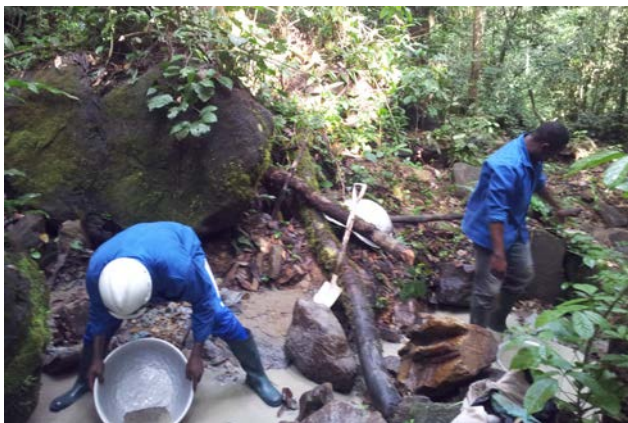
Photos 1 & 2: Stream Sediment and Soil Sampling at Bikala Prospect
