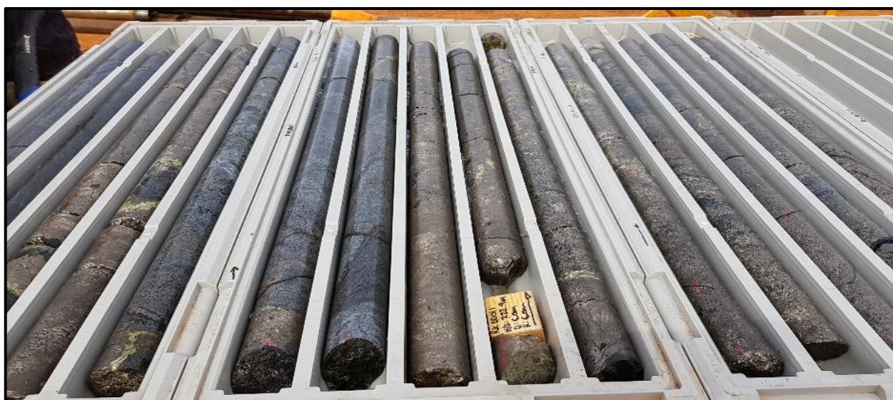
Massive nickel-copper sulphides in RKDD011
