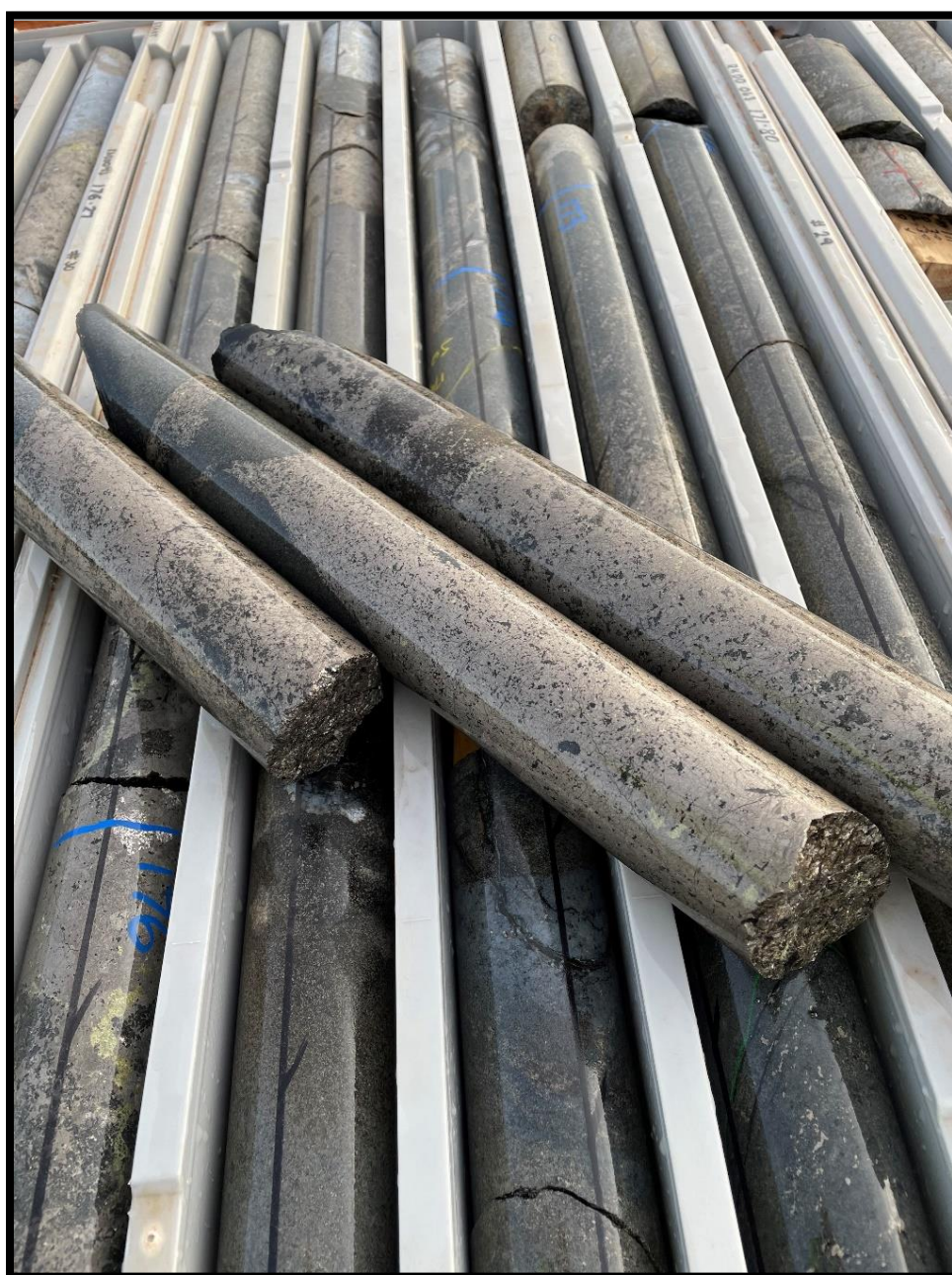
Photo 2: Massive Ni-Cu sulphide from RKDD043 from 181m.
