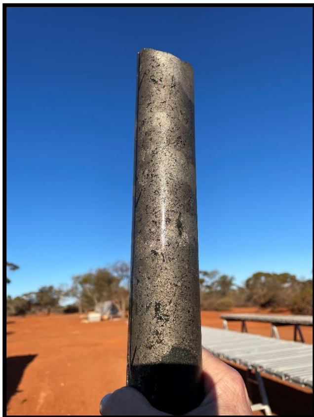
Photo 1: Massive Ni-Cu Sulphide from RKDD044 from 457m
