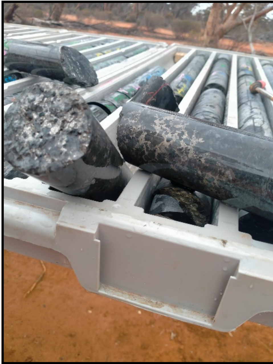
Photo 1: Stringer and blebby pyrrhotite and chalcopyrite sulphides with disseminated graphite within olivine leuconorite from HYDD002 from 415.85m.
