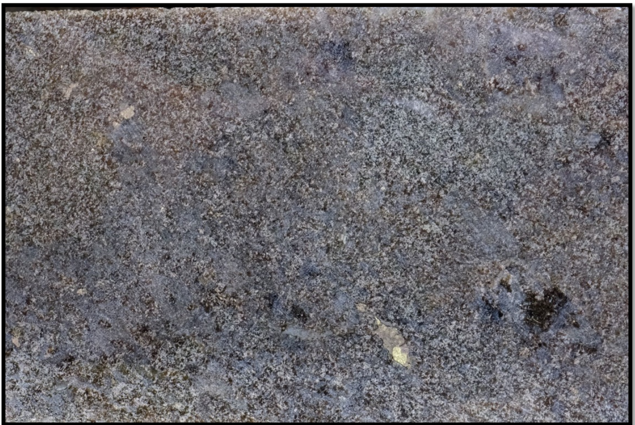
Photo 2: Blebby magmatic sulphides from NODD001 from 96m.
