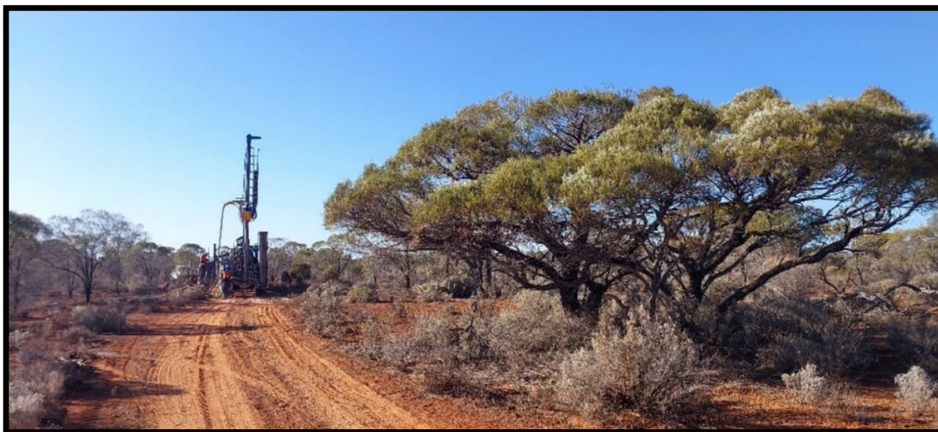
Aircore Drilling at Rockford
