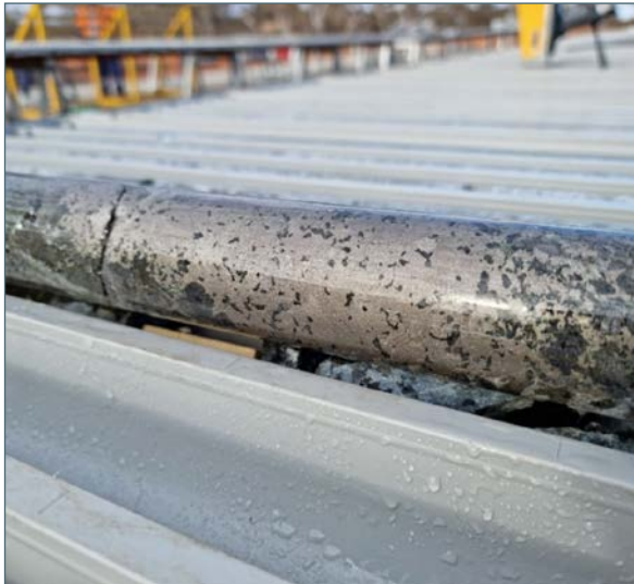
Photo 9: Ni-Cu sulphide mineralisation from OCDD001 from 545.2m and 579.5m at the Octagonal Prospect
