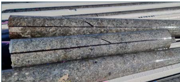
Photo 7: Ni-Cu sulphide mineralisation from RKDD085 from 234m
