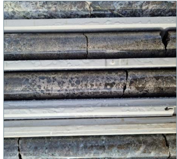
Photo 9: Ni-Cu sulphide mineralisation from OCDD001 from 545.2m and 579.5m at the Octagonal Prospect
