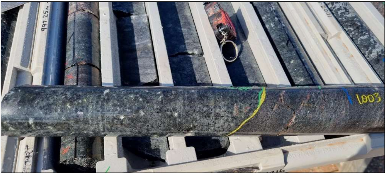
Photo 2: Carbonate contaminated orthopyroxenite and garnet-rich pelite contact from OCDD002 from 1,003m.
