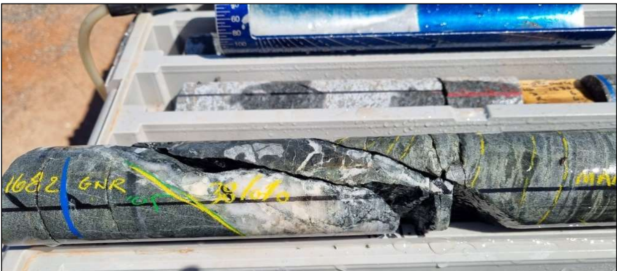
Photo 3: Faulted contact between the OIC and gneissic country rock from OCD004 from 1,682m
