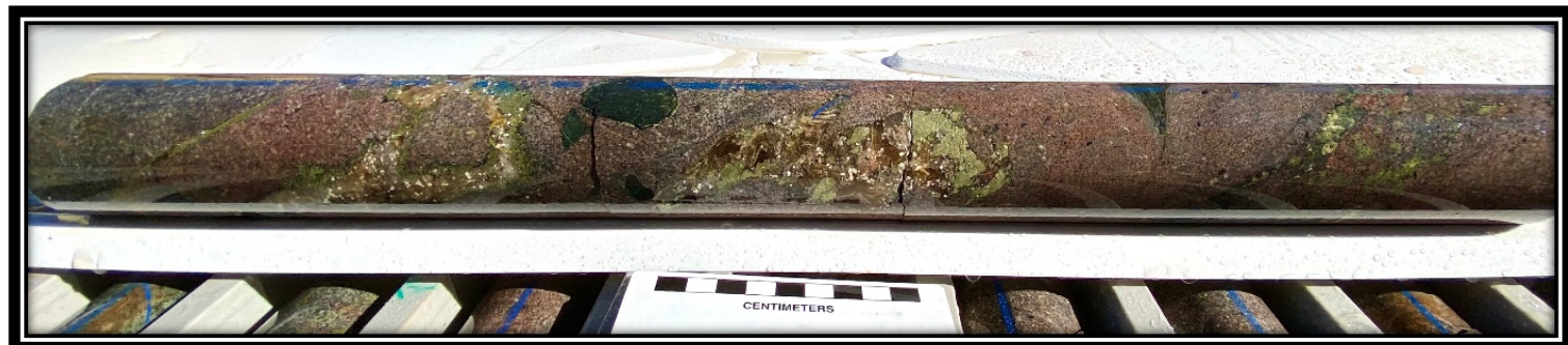
Figure 7 LEFRD267 interval 311 – 311.5m showing chalcopryite with anhydrite, magnesite and strong hematite (red) alteration in quartz feldspar porphyry. The interval also contains a mafic xenolith
