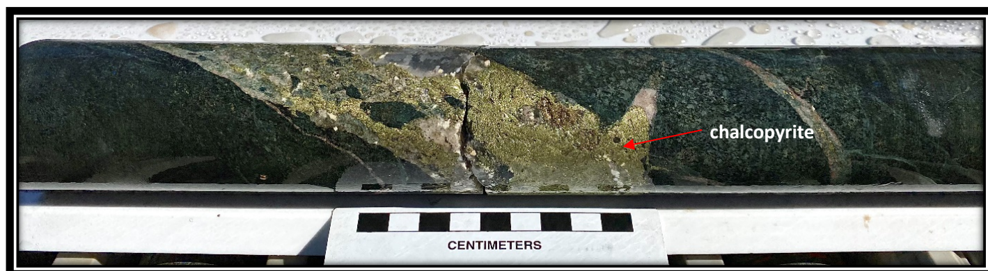
Figure 6 LEFRD267 interval 304.5 – 304.7m showing massive chalcopryrite associated with magnesite and gypsum in basalt.
