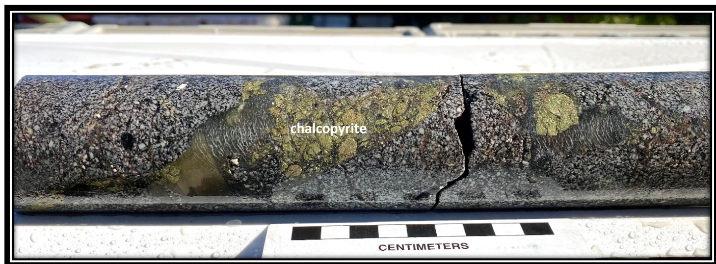
Figure 4 LEFRD267 interval 265.2 – 265.5m showing (gypsum) vein hosted chalcopryrite in quartz feldspar porphyry.
