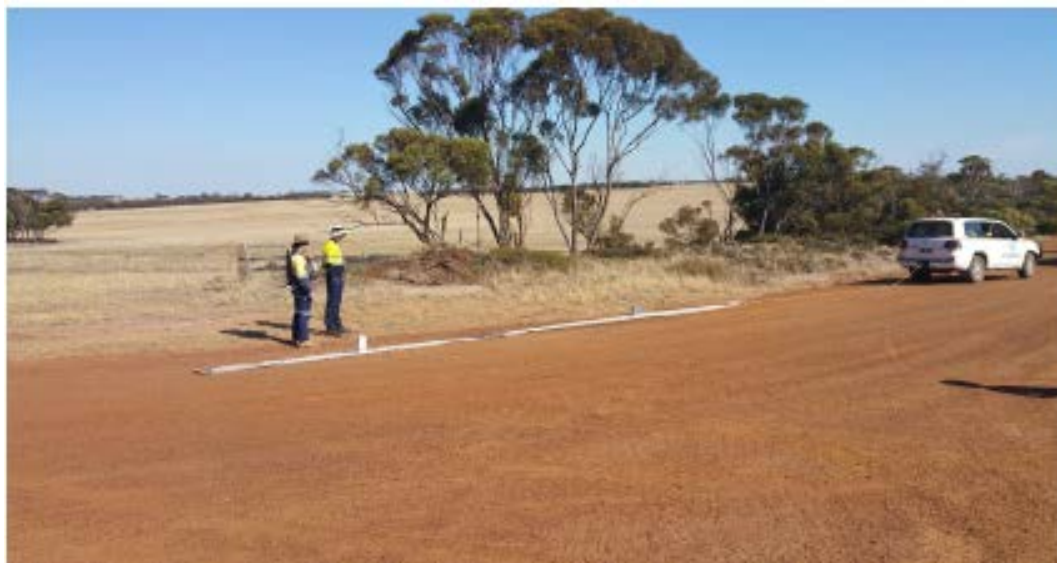
Figure 5 Ground penetrating radar survey underway
