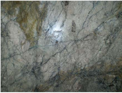
Covellite-bornite vein stockwork and disseminated style mineralisation. Adit 1, north face, Sabang Prospect (1.70% copper, 0.10g/t gold and 4g/t silver).
