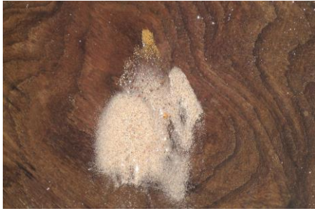
Gold from panning of crushed samples from new veins identified at Layab Prospect.
