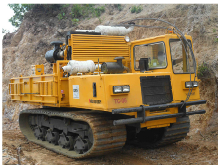
RC rig support unit.
