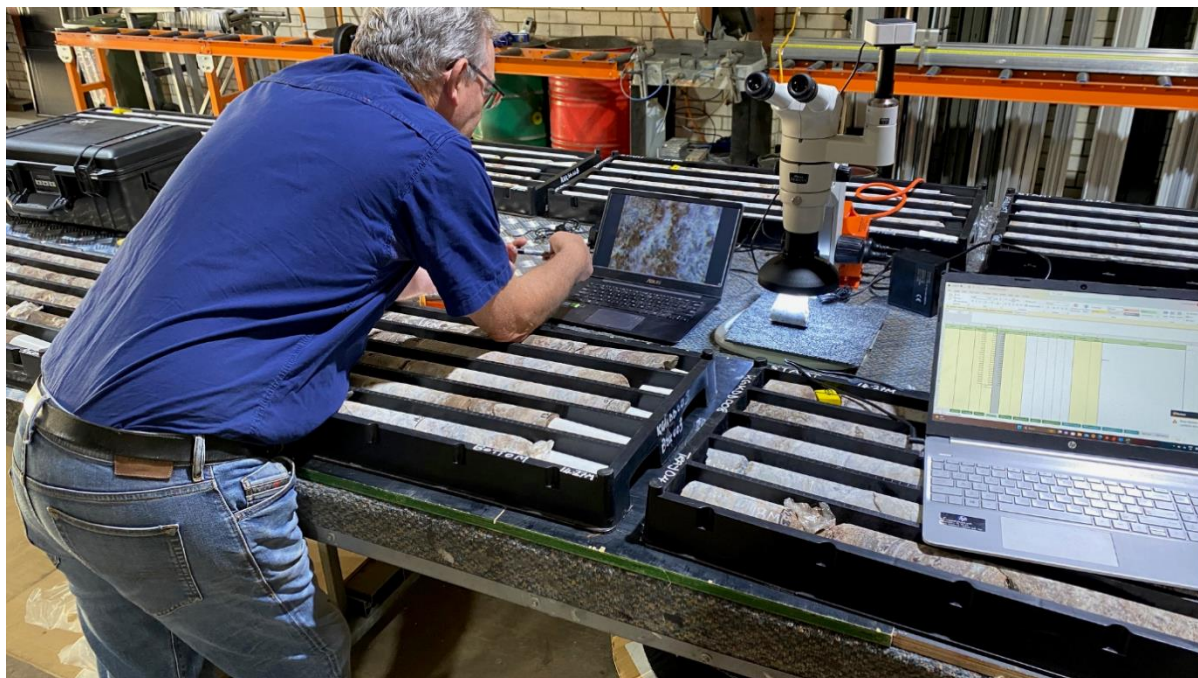
Image 6: Mineralogical Inspection of Kangankunde drill core used in metallurgical testwork.
