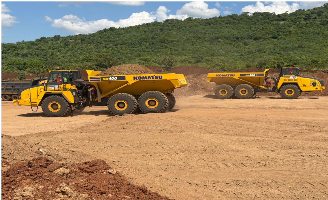
Figure 2: Komatsu HM400 articulated dump trucks hauling fill as earthworks progress across the Kangankunde site, supporting preparation of construction platforms and access routes.
