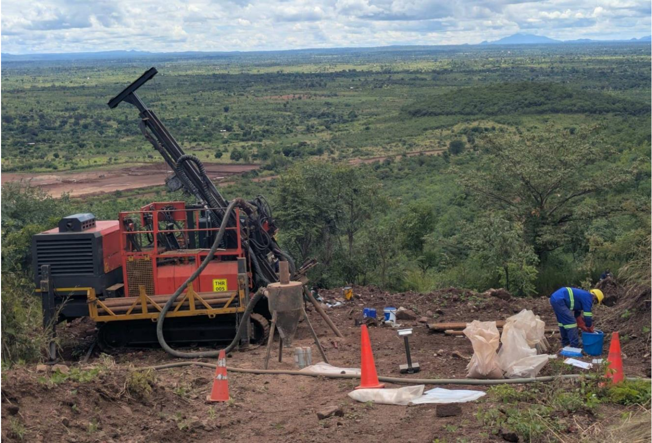
Picture 12. Stage 2 in fill drill rig.
