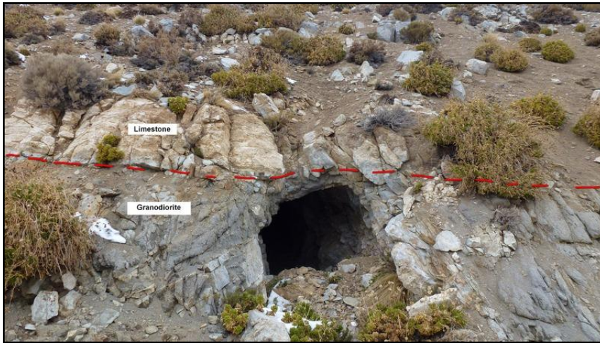
Figure 3: La Demonia adit showing limestone-granodiorite contact
