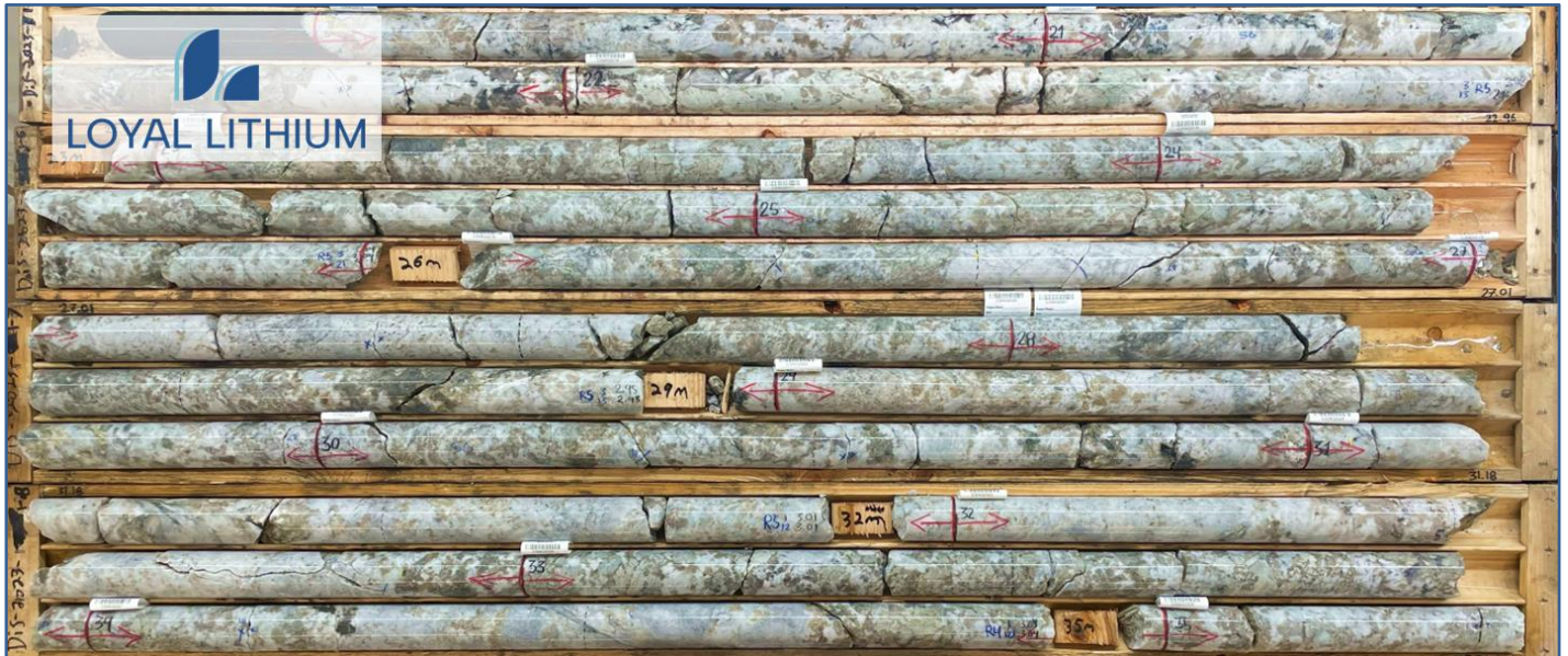
Image 2: Drill core from drillhole DIS23-001 showing significant spodumene mineralisation.
