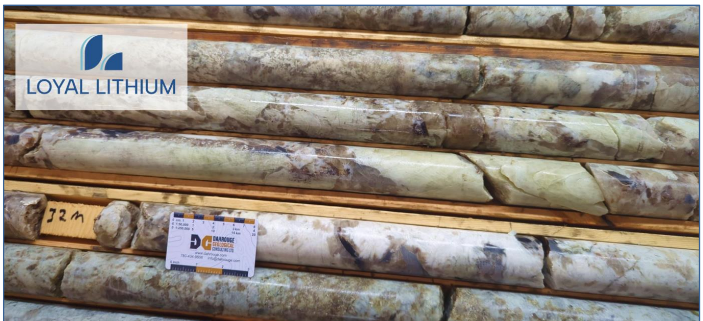
Image 3: Drill core from drill hole DIS23-004, prior to being logged, showing significant spodumene mineralisation.
