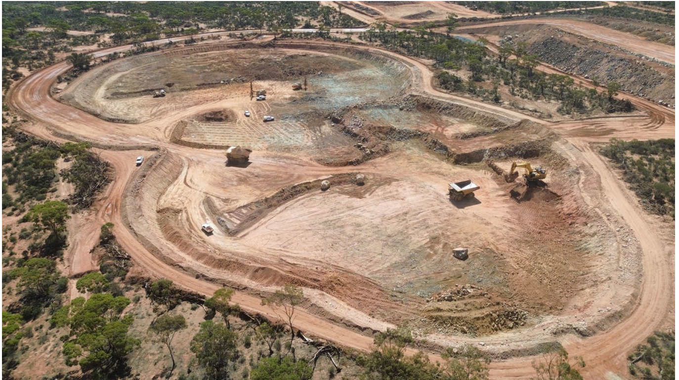
Figure 1: End of April 2026 - drilling & blasting was completed for the 305mRL bench and commenced on the 300mRL bench.
