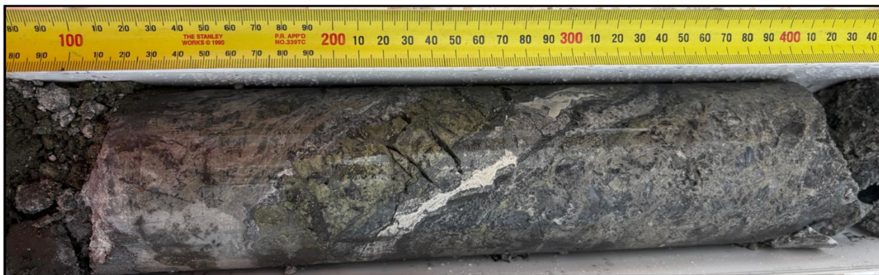
Figure 1: Semi-Massive chalcopyrite (25IRC011D) from 163.2-163.7m – assaying 4.59% Cu.
