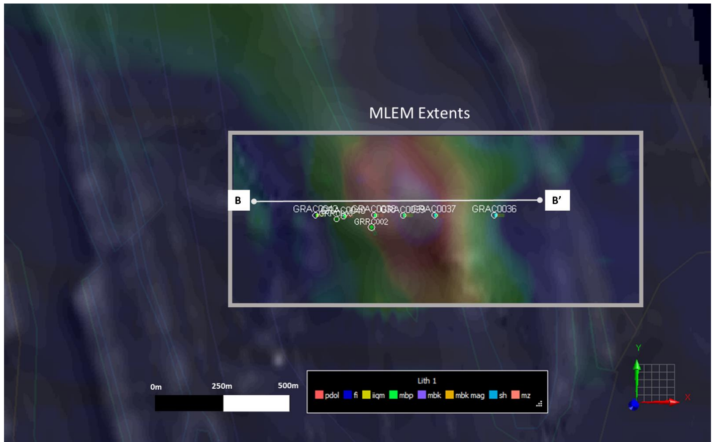
Figure 7. Target B MLEM results showing Ch 10 Image with Peak drillhole positions. Section B-B' marks section positions as also seen on conceptual cross-section.
