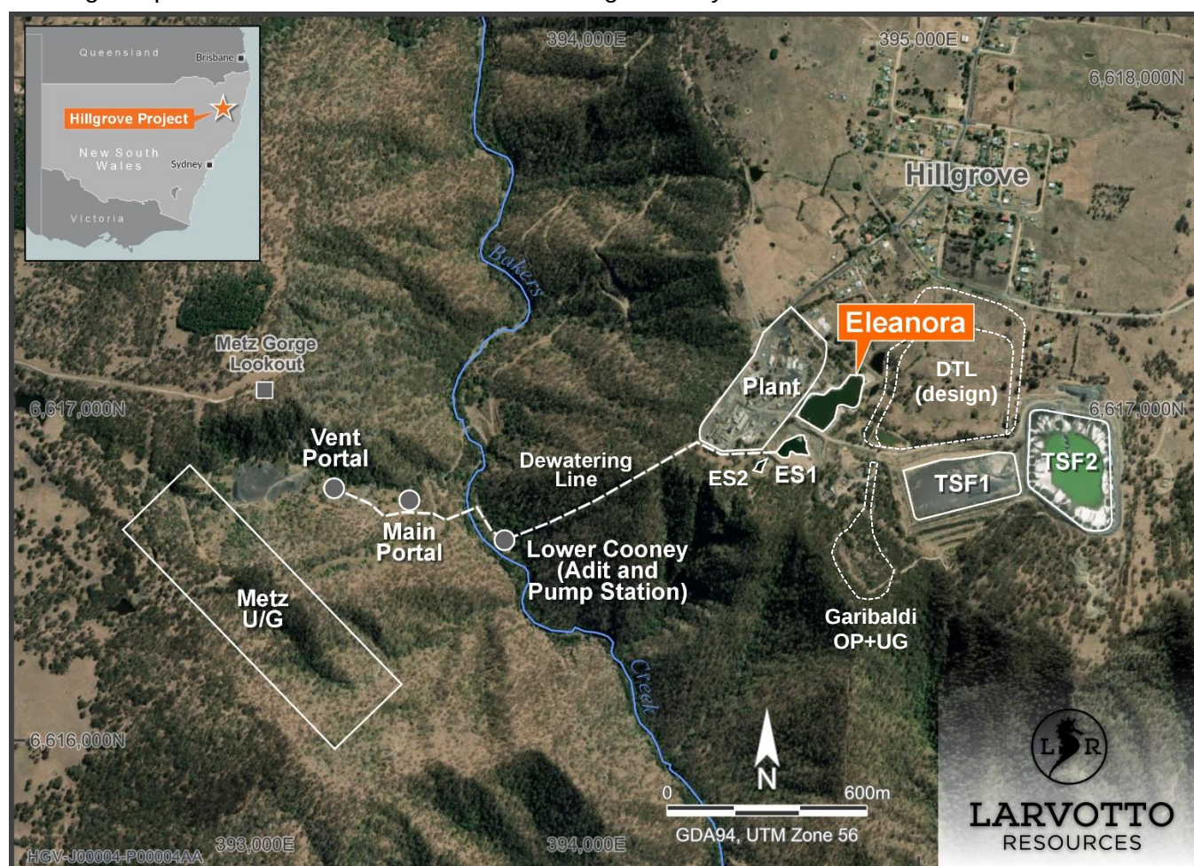
Figure 10 Water management infrastructure at Hillgrove Mine
