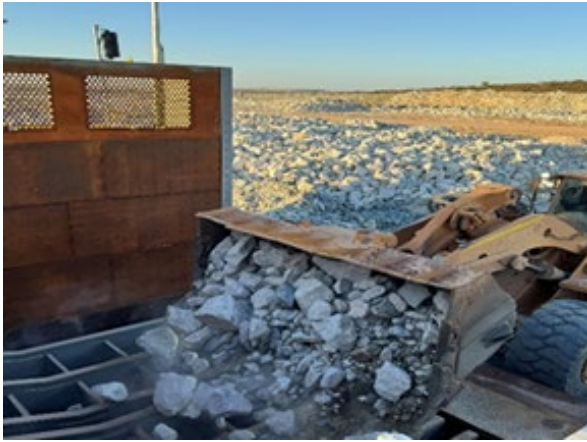
Figure 10: Ore loading into Primary crusher
