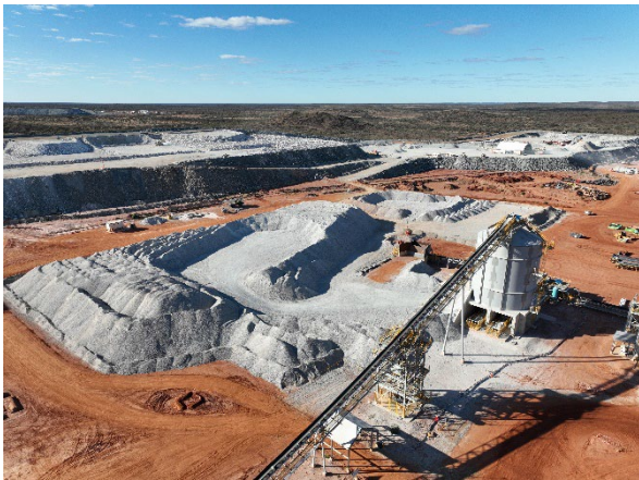
Figure 12: Fine Ore Stockpiles
