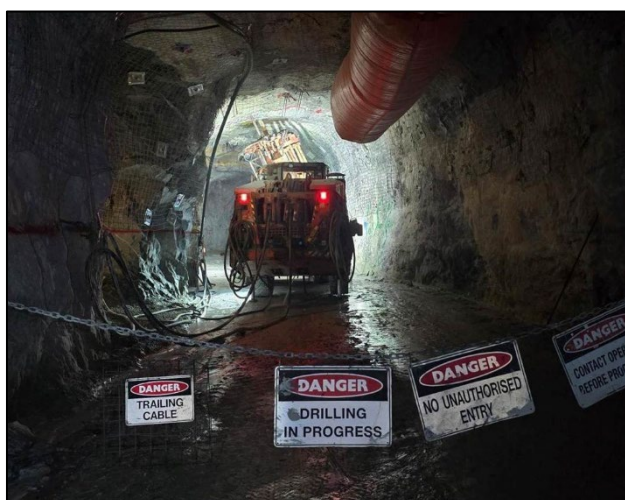
Figure 2: A long-hole drill rig drills upwards into the stope's firing zone
