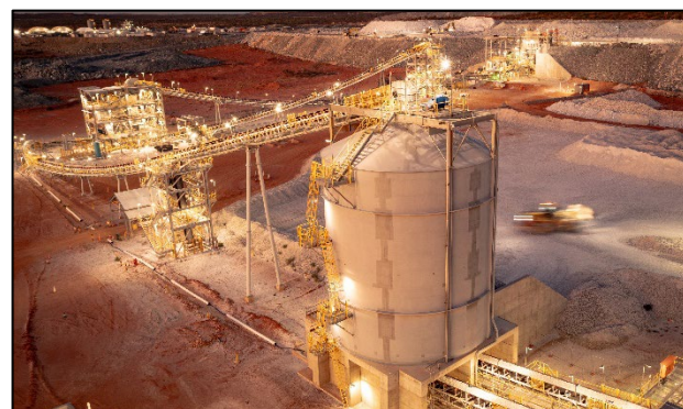
Figure 7: Aerial view of crusher circuit and fine ore bin
