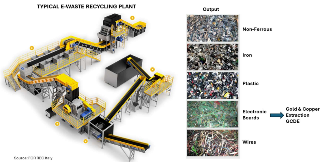
Figure 3 – Typical E-Waste recycling plants separating electronic boards
