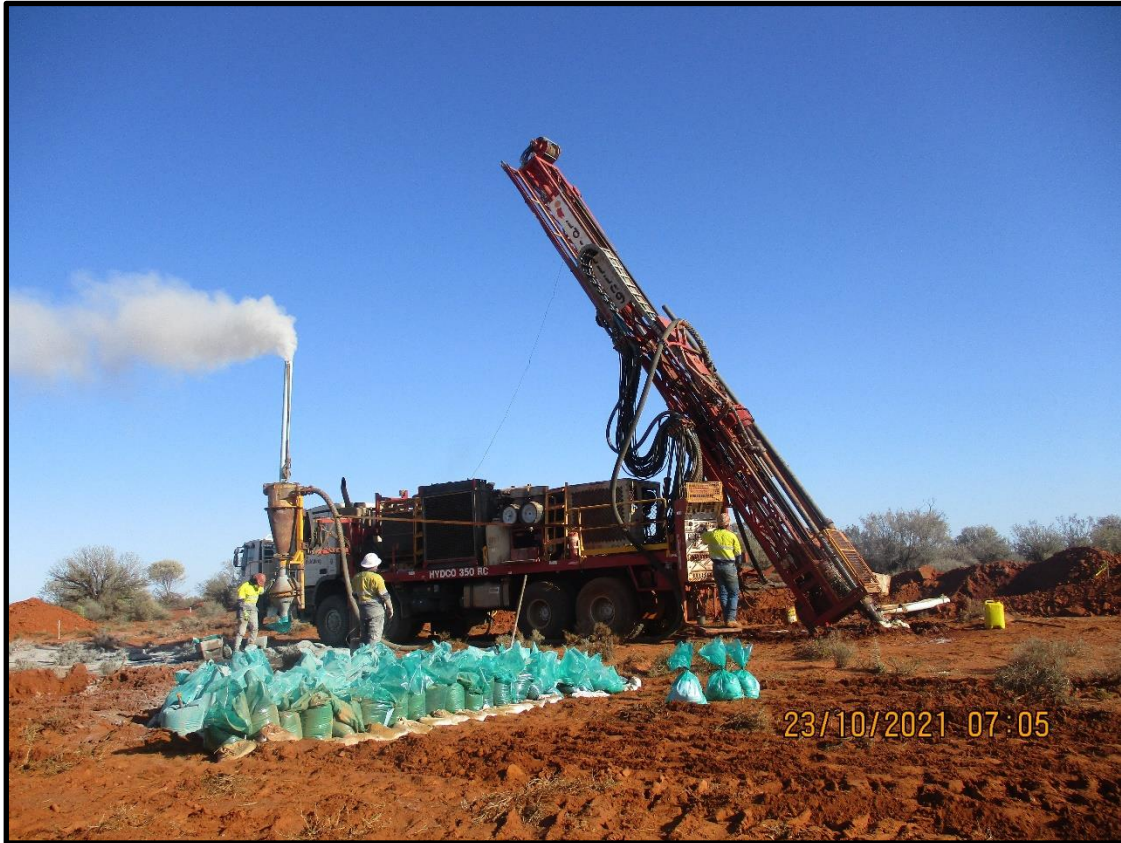
RC Drilling Rig drilling 21CYRC002
