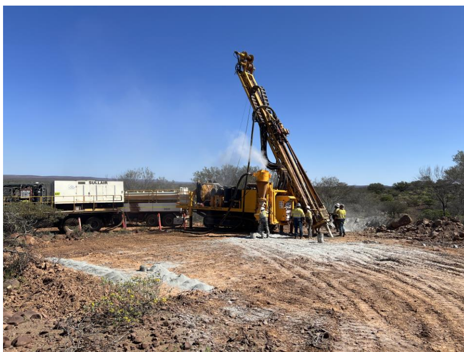
Figure 1. RC drilling underway at Mount Vernon.
