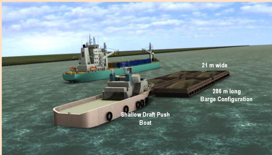
Barge configuration with push boat
