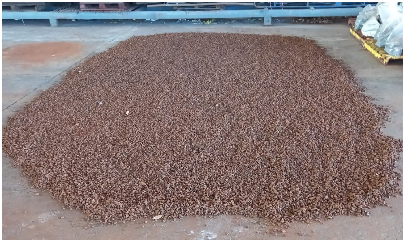
Figure 8 Bulk sample preparation – blending of crushed sample prior to scrubbing tests (top), scrubbed product (bottom)
