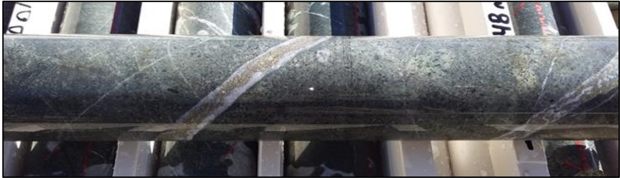
Figure 6. Quartz-carbonate veins (1cm thick) in moderate propylitic (chlorite-sericite-epidote-carbonate-quartz) altered polymictic volcanic breccia (18ATDD012 523m).
