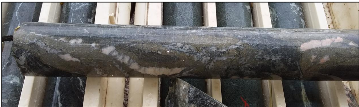
Figure 7. Brecciated quartz-carbonate vein (10 cm thick) with trace of chalcopyrite (18ATDD012 657m) (656-657m; 1.78 g/t Au, 332ppm Cu).
