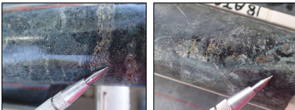
Figure 9. A. Magnetite pyrite vein (18ATDD012 149m); B. Magnetite and pyrite vein with quartz and zeolite (18ATDD012 317m).
