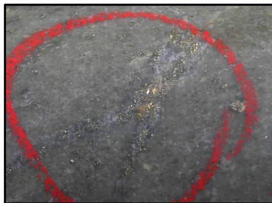
Figure 11: Visible gold in previous Gold Field's 2011 drillhole BYRCD004: 0.3m at 2.07 g/t Au, from 248.6m – silica altered andesitic polymictic breccia with carbonate-quartz-pyrite-galena
