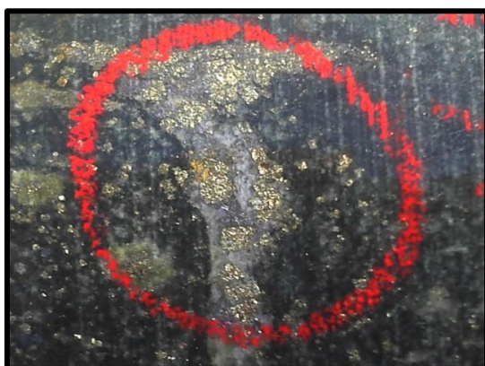
Figure 10: Visible gold in previous Gold Field's 2011 drillhole BYRCD004: 0.35m at 4.35 g/t from 245.6m
