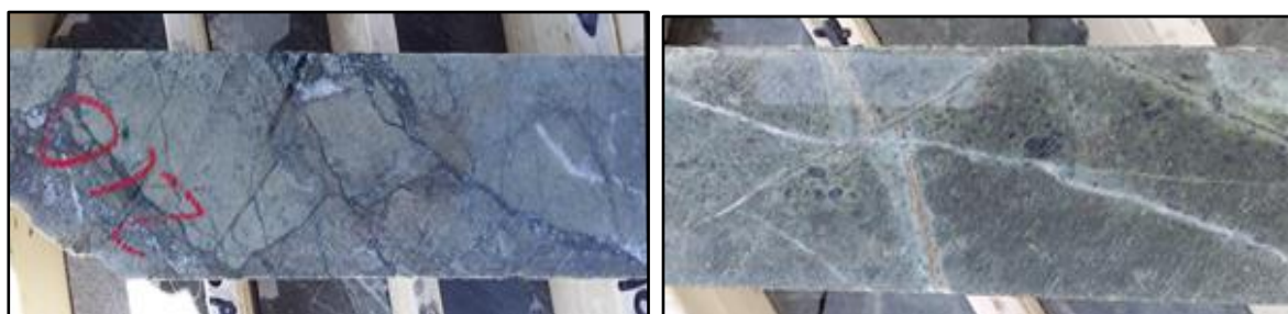
Figure 4. A. Hydraulic breccia of intensely altered (silica-sericite+/-albite) porphyritic diorite. (18ATDD012 210 m); B. Intense carbonate, chlorite, +/-epidote, +/- pyrite veins with alteration selvage of sericite-epidote-carbonate.
