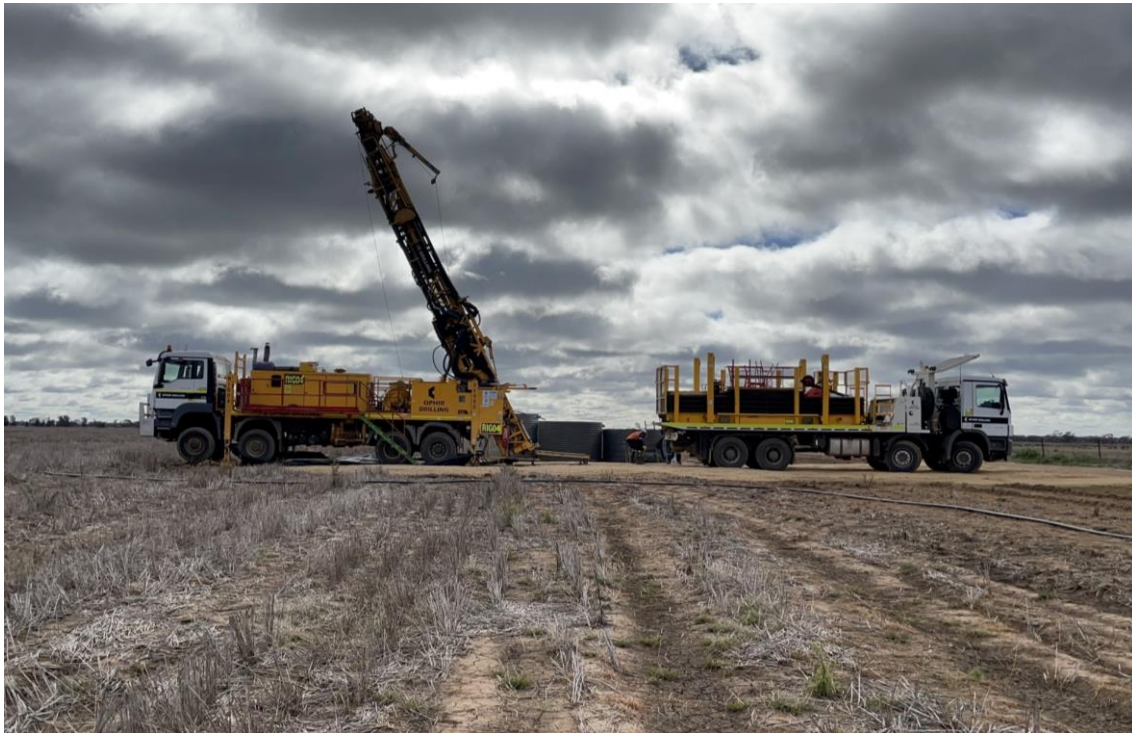
Figure 1. Diamond drill rig set-up at the site of the first drill hole (22MYDD414) at the Corvette Prospect.
