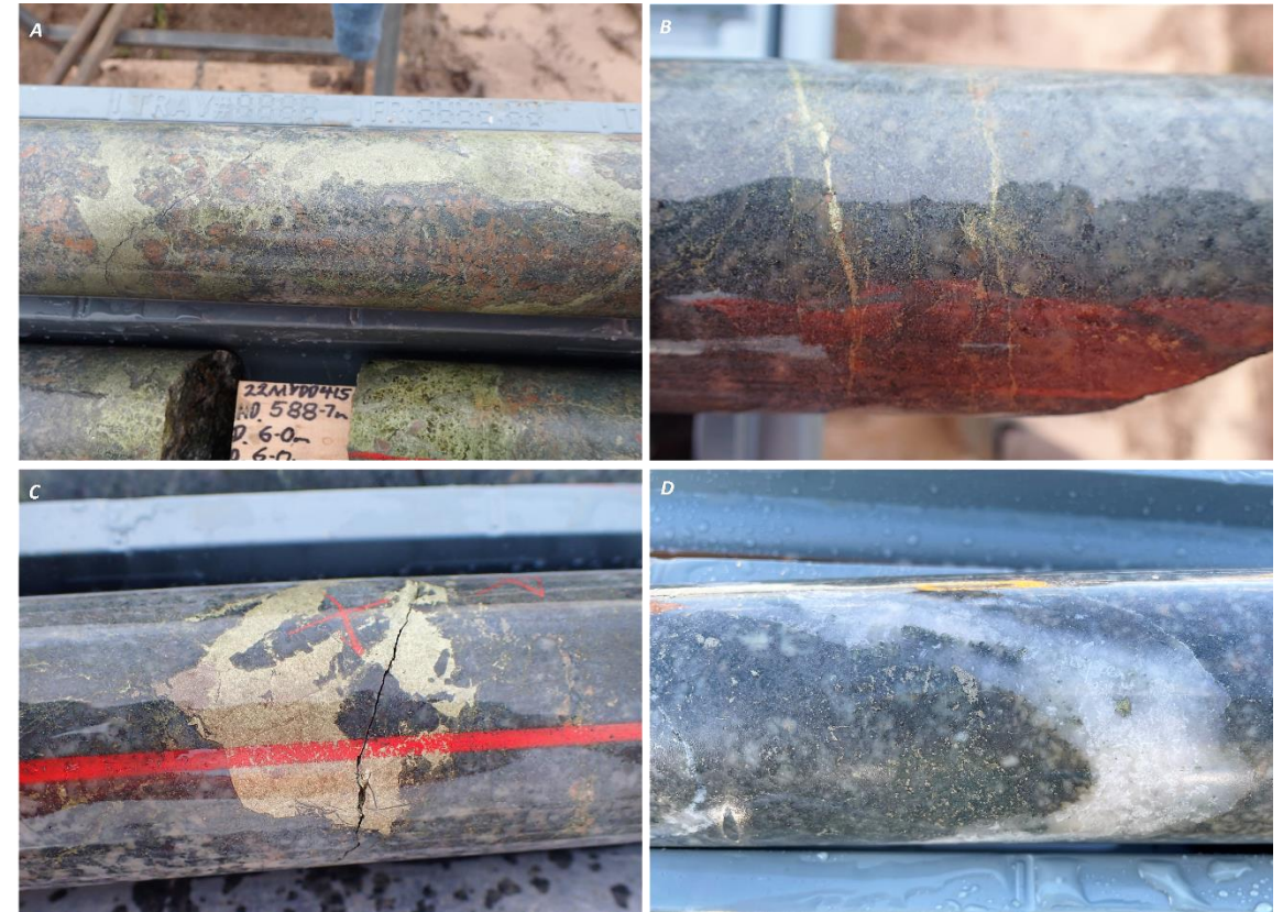
A) Chalcopyrite (yellow) and epidote (green-yellow) within a K feldspar altered polymict breccia from 588m; B) thin chalcopyrite-pyrite veins cross-cutting a pervasively chlorite-altered diorite from 595.2m; C) brecciated, chlorite-altered diorite strongly infilled with chalcopyrite and lesser pyrrhotite from 730.5m; D) chlorite-altered diorite with abundant disseminated pyrite, cut by quartz-carbonate veins with minor chalcopyrite from 810.2m.
