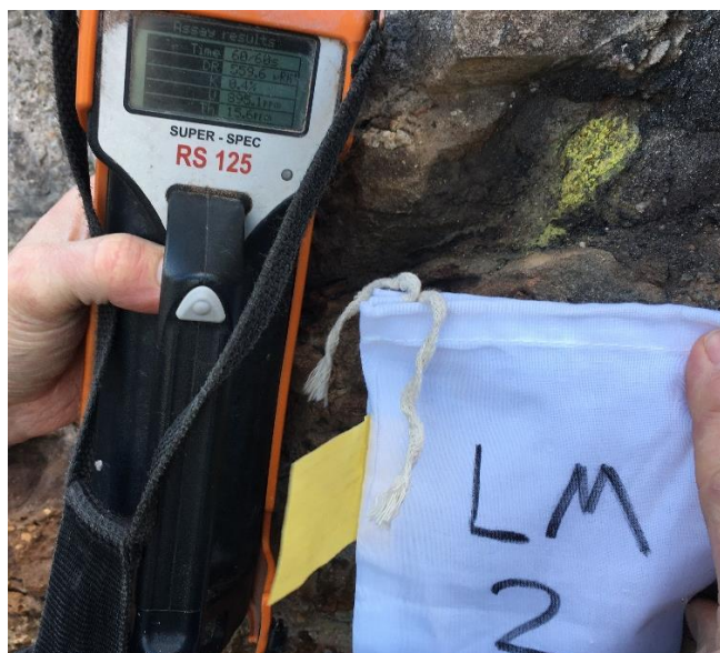
Figure 1: Carnotite in dark-coloured beds bounded by sandstone (sample LM2)
