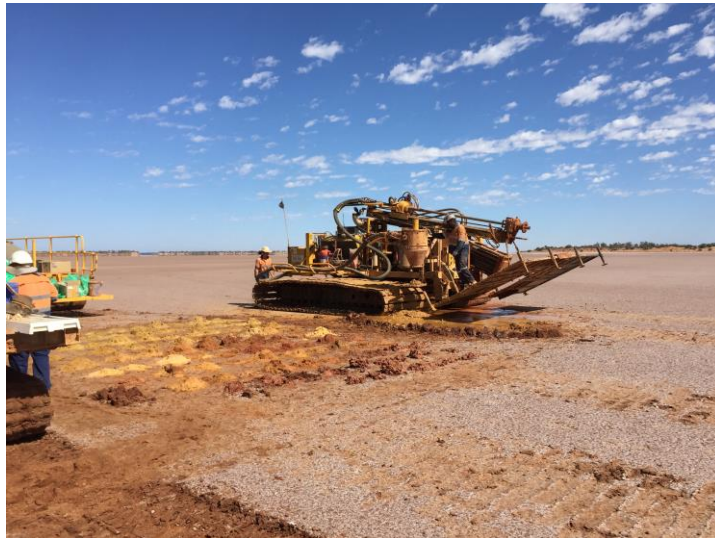
Figure 4: Lake Aircore Rig operating Bindah Extended
