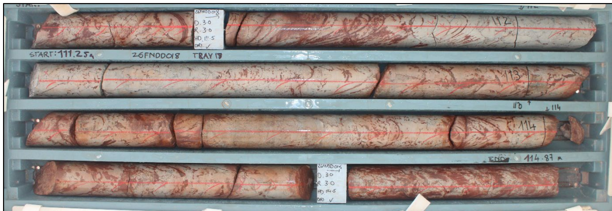
Plate 1: Drill core from 26FNDD018 (111.25m to 114.87m) showing oxidation and strong albite (bleached) alteration typically associated with gold mineralisation at Fortitude North (photographed dry)
